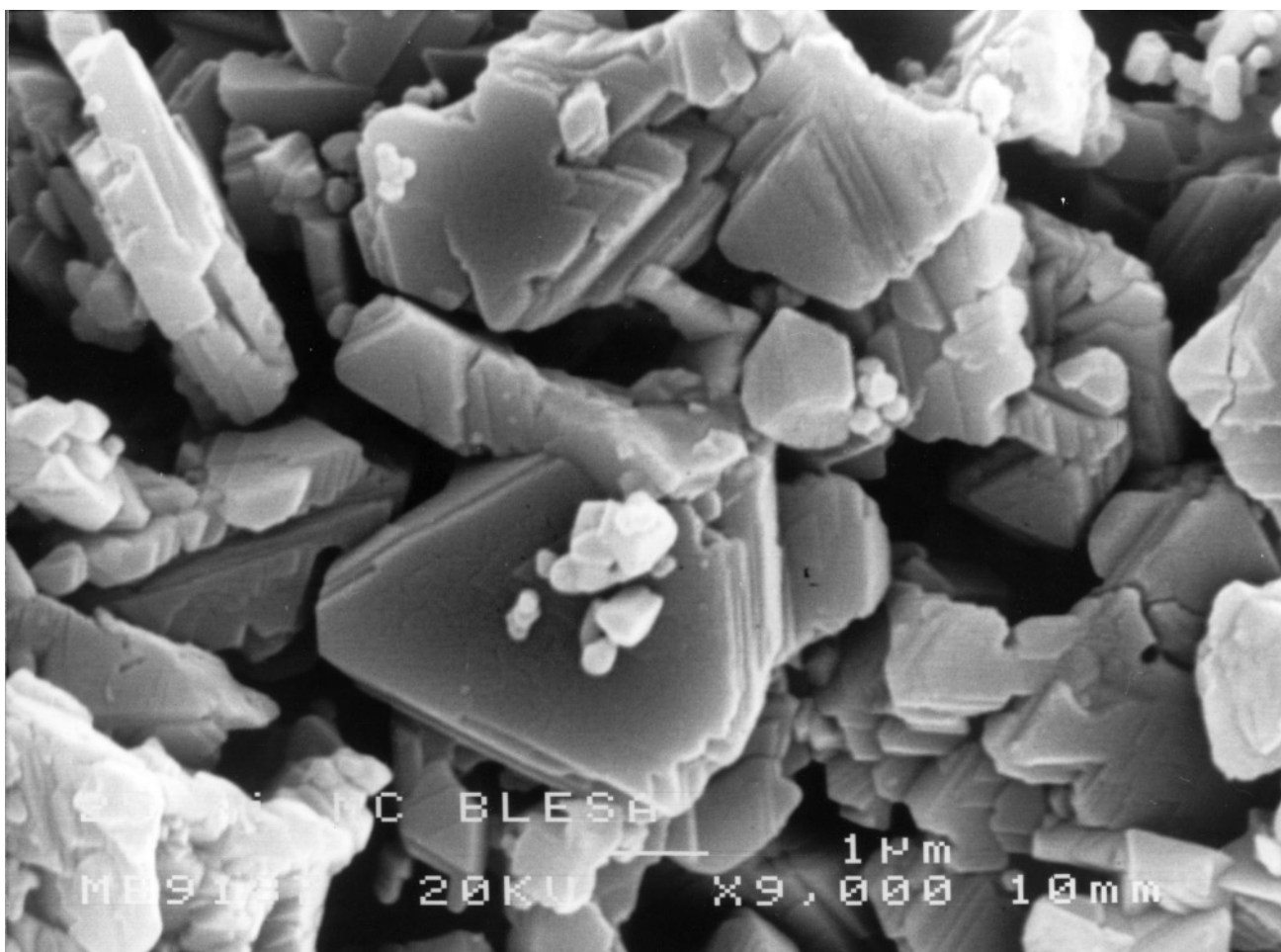
FIG. 1. Scanning electron micrograph of the Ni-Fe spinel-like compound. The shape of the particles of the precursor \alpha - \text{NaFeO}_2 is retained.
